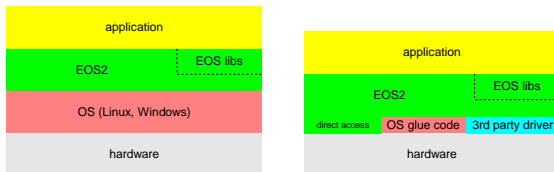
Fig. 1. Layer model of EOS2 abstraction (left with high level OS e.g. Raspberry Pi, right with rudimental OS e.g. Arduino)
